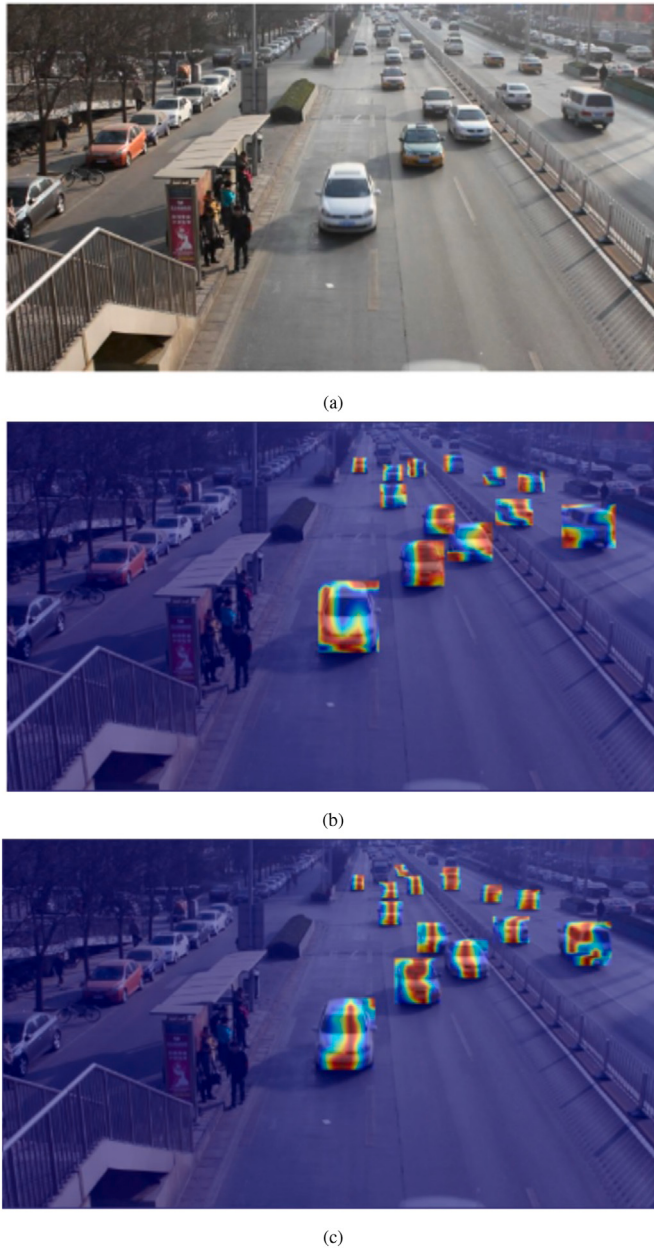
Fig. 20. Heatmap comparison showing (a) original image, (b) PSO-YOLOv7x with focused attention (82.1% ACI), and (c) YOLO-AL baseline (71.5% ACI). Quantitative metrics in Table X confirm PSO-YOLOv7x achieves 13.8% higher attention concentration and 13.3% better background suppression.
