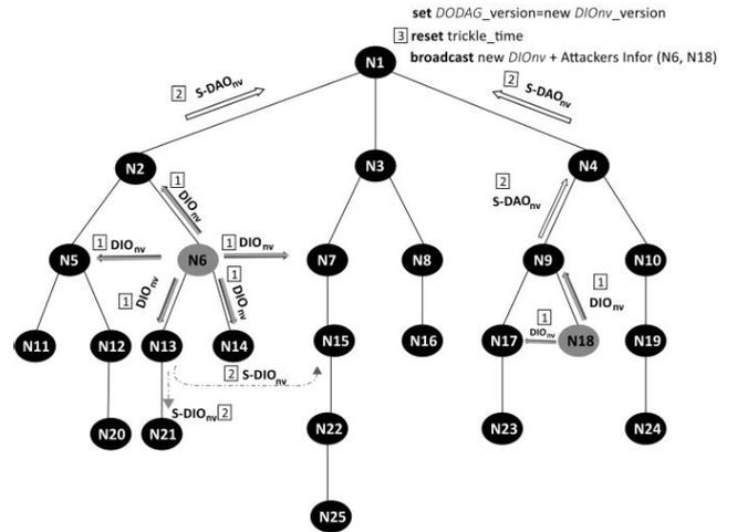
FIGURE 7. Example of a composite VN attack scenario with two attackers (N6 and N18).
