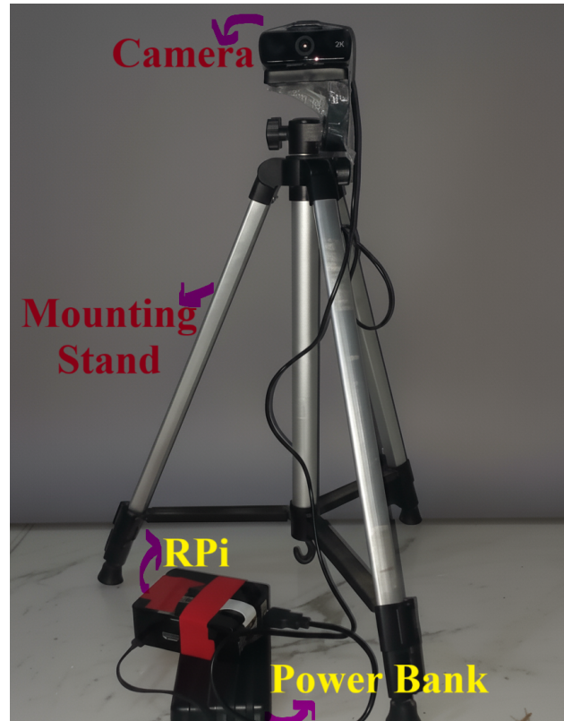
Figure 4. Edge device setup used for real-time fire and smoke detection. The configuration includes the Raspberry Pi 5, camera module, power supply.
