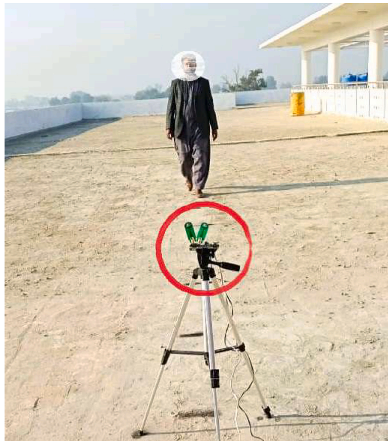
Fig. 2. Subject moving toward P410 radar mounted on stand and encircled red.
